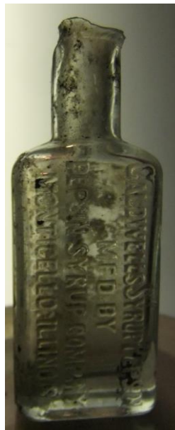
Rejected CALDWELLS SYRUP (front view), note that the lips were not finished – photo courtesy Tom Kennedy-Jansen
